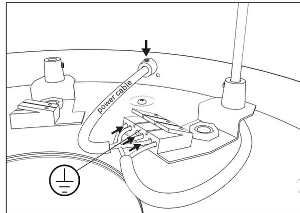
Lead the power cable into the ceiling plate and make sure the cable relief is tightened.
