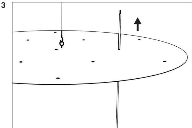
Lead the cables through the cover plate.
