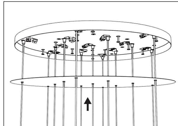
Attach the cover plate to the ceiling plate by carefully sliding it up and let the magnets fixate the cover plate to the ceiling plate.
