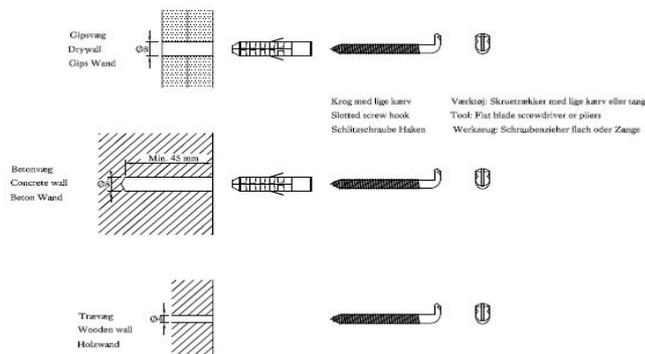
Template for drilling for mounting screws.
